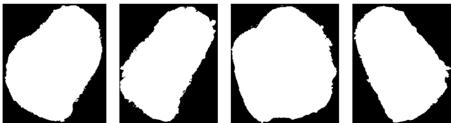
Fig. 3 Binarized sand particle scans, obtained with a confocal microscope.
